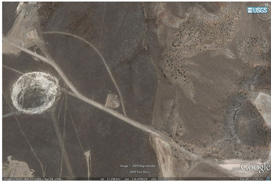
Figure 81. Google Earth image of the crater of the UNE Boxcar (left), the nation's first megaton nuclear device detonated April 26, 1968, and Boxcar Bluff (right), cliffs of densely welded tuffs shattered by Boxcar ( Figure 82 ). The crater is about 400 m in diameter.
